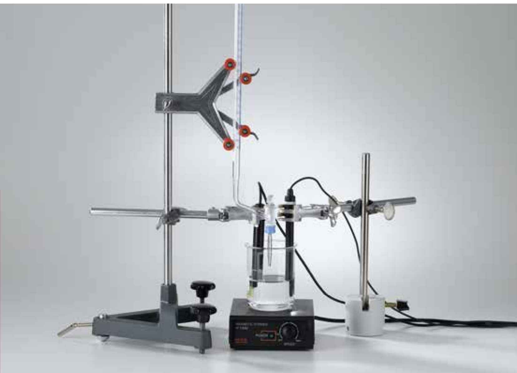
Conductometric titration of a hydrochloric acid solution with pH measurement (C3.5.2.2)
